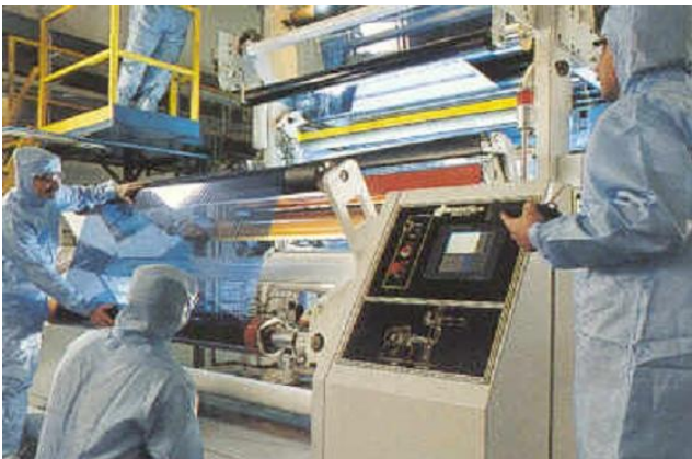
Figure 2: Coating and lamination of two polyester films in a clean room during window film manufacture
