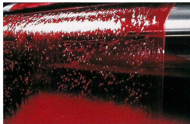
Figure 5: Deep dyeing of polyester film – the finished film must be a high clarity, low distortion product
